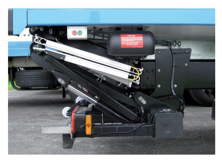
The MBB F 1500 L is a lightweight, 2-cylinder tuckunder tail lift, with an aluminium platform capable of lifting 1500 kg at a 600mm load centre. Its folding platform stows under the vehicle chassis, providing clear access to the rear of the vehicle when required.
