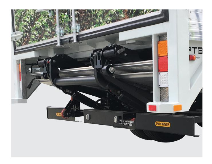
The double-folded MBB F 1000 L is a light, foldable two-cylinder tail lift which is mounted underneath the rear of the vehicle. Its 1000 kg lifting capacity ensures secure handling of pallets and trolleys alike. The MBB F 1000 L offers stability due to two lift cylinders and two parallel arms. Ground tilting of the aluminium platform is mechanical.
