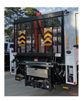
The MBB C 750 SM tail lifts platform is specially designed for Australia and is suitable for small vehicles up to 7.5 tonne gvm. The lift features robust four-cylinder lift mechanism with an overall lift weight of only 230 kg. Available platform sizes 1300 mm height with 1900 and 2200mm width options. A three-piece screwable, underrun bumper is standard. Boltable mounting brackets enable quick installation to virtually all types of chassis.
