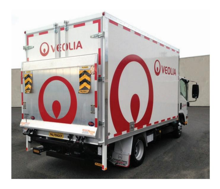
The MBB C 750 S tail lift is specially designed for small vehicles up to 7.5 tonne gvm. The lift features a strong, lightweight aluminium or steel mesh platforms and a robust four-cylinder lift mechanism with an overall lift weight of only 224 - 230kg (dependant on platform) A three-piece screwable, under-run bumper is standard. Universal mounting brackets enable quick installation to virtually all types of chassis.
