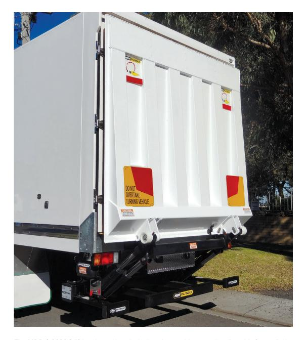
The MBB C 3000 S lift has been cleverly designed to provide exceptionally stable four-cylinder operation capable of lifting goods up to 3000 kg, making it ideal for the transportation of the heaviest loads. It is available with either a steel or aluminium platform with a load centre of 1000 mm. A powerful, low-noise powerpack in the square main beam reduces noise during loading or unloading to a minimum.
