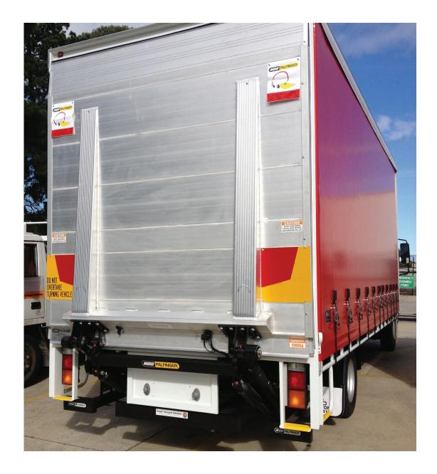
Lifting a full 2000 kg, the MBB C 2000 S is the tail lift of choice for the food and drink distribution industry. Its reliable and heavy duty four-cylinder lift mechanism is available with a wide variety of steel or aluminium platforms, up to a maximum height of 2600 mm.
