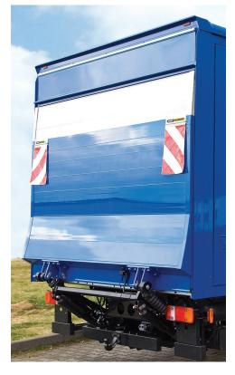
The MBB C 1500 S traditional cantilever lift is designed for heavy duty use with 1mt load centre and exceptional performance rating this lift is perfect for palletised freight deliveries. Available with aluminium platform, this model features four-cylinder technology and is suitable for a wide range of floor heights and ideal for larger vehicles.
