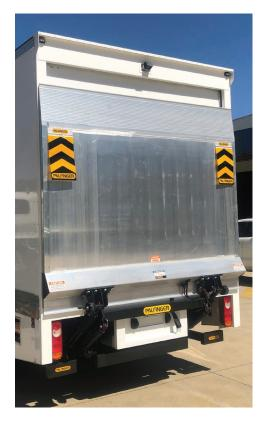
The MBB C1000 S traditional cantilever lift is designed for heavy duty use and is extremely robust and dependable for day-to-day use, with an exceptional performance rating. Available with aluminium platform, this model features four-cylinder technology and is suitable for a wide range of floor heights.
