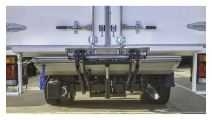
The FTK6OOE is a compact tail lift with a foldable platform and a loading capacity of up to 6OOkg. This results in an optimal weight-to-capacity ratio. The low weight is achieved with an aluminium platform and innovative design. The folding platform stows under the vehicle chassis and is simple to operate and quick to install. Comes standard with mechanical auto-levelling for increased stability when lifting larger loads.
