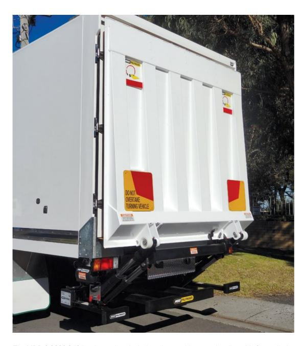
The MBB C 3000 S lift has been cleverly designed to provide exceptionally stable four-cylinder operation capable of lifting goods up to 3000 kg, making it ideal for the transportation of the heaviest loads. It is available with either a steel or aluminium platform with a load centre of 1000 mm. A powerful, low-noise powerpack in the square main beam reduces noise during loading or unloading to a minimum.
